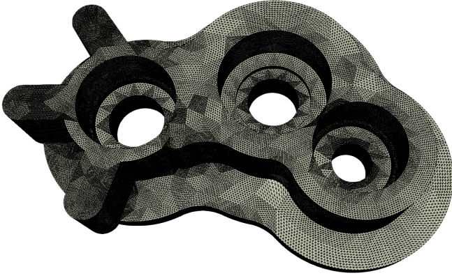
Figure 8: Geometry and BE mesh of the pump casing model with 1 728 508 DoFs.
