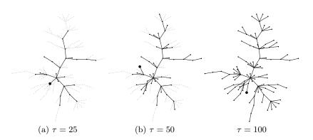
Fig. 5. Growing a tree by preferential attachment  $(n = 100, \kappa = 1)$ . The node  $v_{\tau}$ , being added to the tree at time step  $\tau$ , is emphasized (larger circle). Dotted edges at time steps  $\tau = \{25, 50\}$  are a visual aid representing edges that are yet to be added in the tree until the order-limit (n = 100) is attained.
