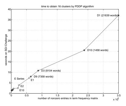
Figure 9: Times for the PDDP algorithm on an SGI versus number of nonzeros in term frequency matrix, for both E and D series with 16 clusters. The D experiments had 2,340 documents and the indicated number of words, and were constructed just like the corresponding E experiments in Table 1.
