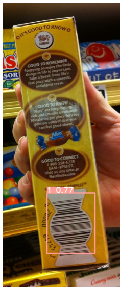
Figure 3: Barcode object detector
