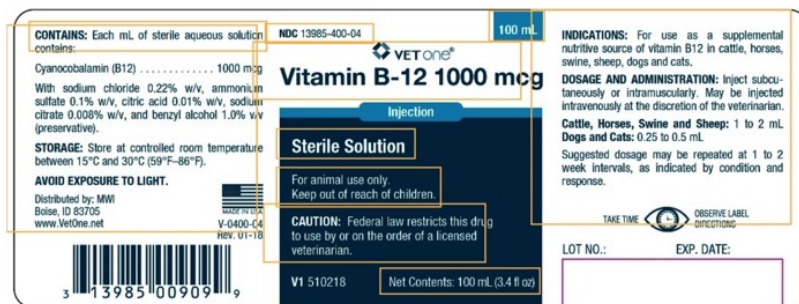
Figure 8: Example of a layout analysis by the fine-tuned model
