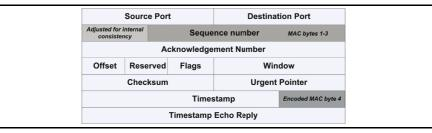
**Fig. 4.** The TCP SYN packet after steganographic embedding. The "internal consistency" adjustment in the sequence number is performed to keep the modified sequence number consistent with what Linux is expected to produce.
