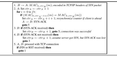
**Fig. 2.** The pseudocode for SILENTKNOCK. A is the server, B is the client,  $ctr_P$  is a per-IP-address counter maintained by principal P, k is a value derived from B's IP address and a symmetric key shared between A and B, m is a TCP flow identifier, and ft is a failure-tolerance parameter.
