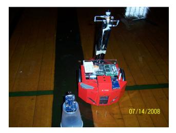
Figure 3: An Acroname Garcia robot visiting a sensing mote. Note the single board computer on the robot under the clear lid and the mote connected to the robot's computer.
