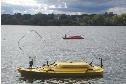
Fig. 1. The robotic systems used in field experiments. The 2-meter long boats were designed to track invasive fish autonomously. Each is equipped with wireless communications, directional antenna used as bearing sensors, a navigation suite, and computing hardware. Our algorithm was implemented on this system which was shown to localize targets with small uncertainty.
