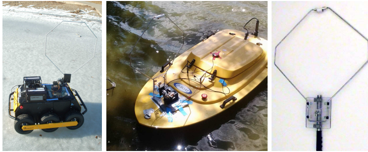
Figure 1: The robots designed for tracking fish during the winter (left) and summer (middle). The direction-sensitive antenna mounted on the robots (right). The bearing to the target can be estimated by rotating the antenna every \alpha degrees. The bearing corresponding to the maximum signal strength is taken as the true bearing. Thus, the uncertainty is at most \alpha .
