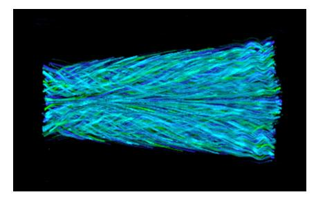
Color Plate 1: A volume rendered image of a 3D flow dataset generated using volume LIC. Color variations are used to differentiate the individual streamlines and to facilitate the conscious direction of focused attention to subsets of these lines. Depth discontinuities are explicitly indicated by means of a locally-defined 3D "halo" that impedes the visibility of underlying texture elements in the vicinity of overlying lines.
