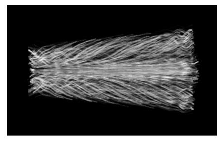
Figure 1: A volume-rendered image of a 3D texture generated by volume LIC from an input texture of evenlydistributed random point samples, premultiplied by a function of the velocity magnitude. Shading is computed as a function of the angle between the flow direction and the light direction, as motivated by [27], [2], and others. Note, nevertheless, the lack of a clear indication of the local depth order relations between overlapping and adjacent lines.
